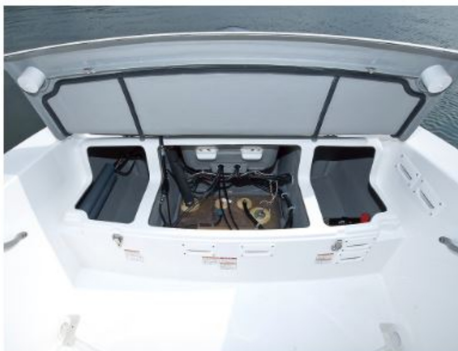
Fixed fuel tank (70L) and battery space
