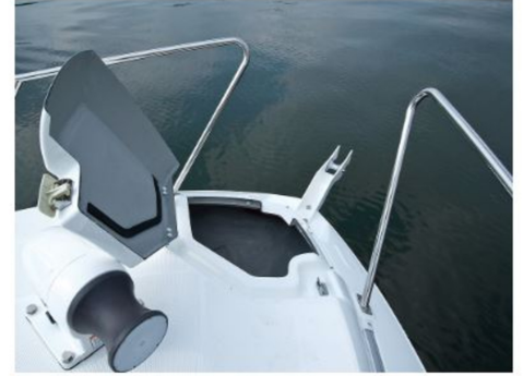
Bow locker / anchor winch
